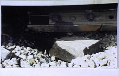
Photo 2. View of the POD, and the East end rail segment of the 14 foot 11 1/2 "plug" rail
