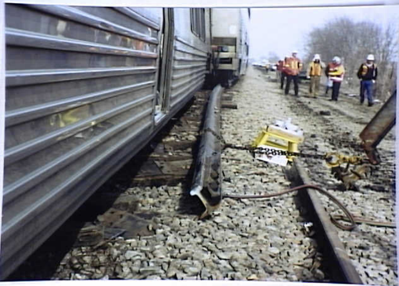
Photo 3. View of the rail end at the POD being pulled out for a closer inspection
