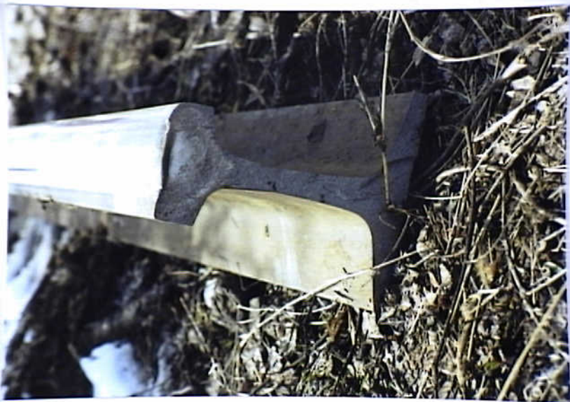
Photo 5. Rail end view of the matching rail face from the POD, and middle segment of the 14 foot 11 1/2 inch "plug" rail
